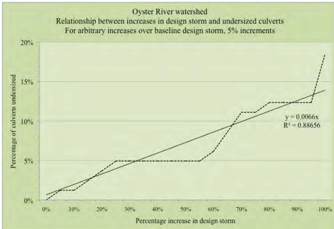
Figure III.c.4 The relationship between arbitrary percentage increases in the design storm, and the percentage of undersized culverts
